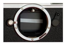
As you can see, one of the shutter slats is 18% gray to reflect light to the bottom mounted meter cell.
