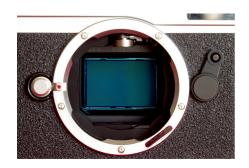
More importantly, neither the M8 nor the DMR have anti-aliasing filters over their sensors. AA filters reduce the moiré patterns caused by regular geometric patterns interfering with the regular spacing of the pixels. But they also reduce the ability of the sensor to capture fine detail.
